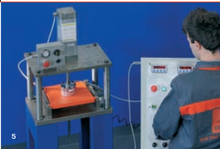
Fig. 4/5 Par. 4.6 FLEXION TEST ON RUNGS OR ON STEPS OR ON PLATFORM
